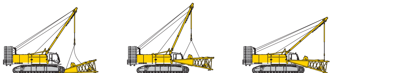
Unloading and assembly of boom foot
